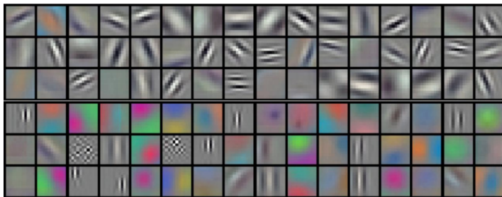
Figure: “96 convolutional kernels of size 11 \times 11 \times 3 learned by the first convolutional layer on the 224 \times 224 \times 3 input images.” [KSH12]
